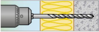
1. Drill a hole  $\varnothing 10$  mm through the insulation into the wall material. Drill depth in concrete min. 40 mm.
