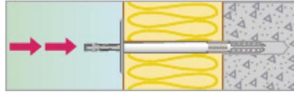
2. Push in the Insulation holder until the washer rests against the insulation. Now knock in the pin. For soft insulation, the extra washer is pushed onto the insulation holder before installation.
