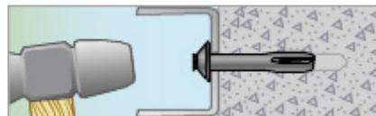
1. Place the detail in position. Drill through the studs straight into the underlying concrete. Drill dimension according to the tabel below.
